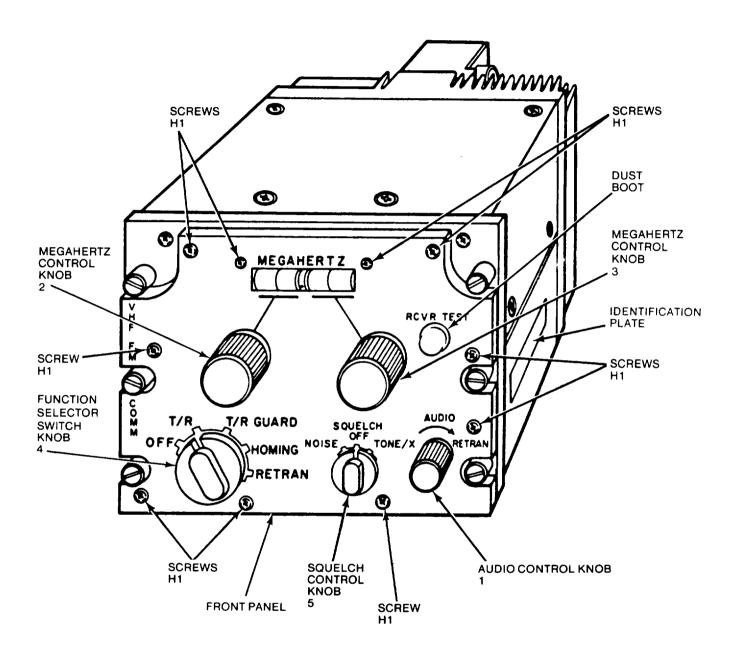
Figure 1. Location of Front Panel Controls Attaching Hardware
