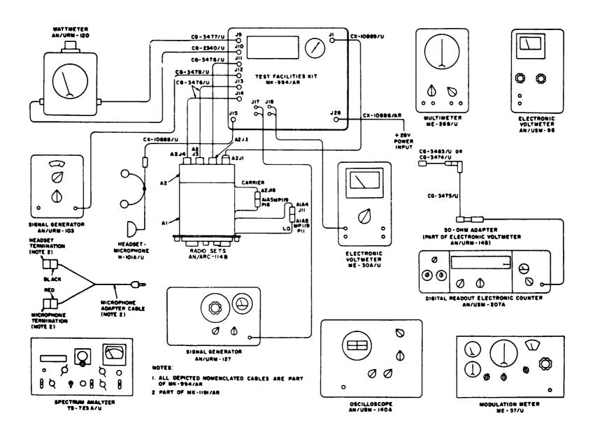
Figure 3. Radio Set Test Setup Diagram
