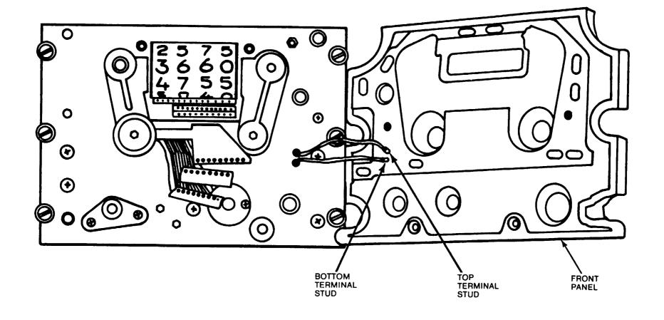
Figure 2. Remove/Install Front Panel From Radio Set
